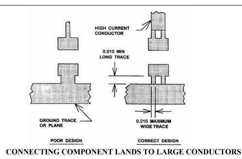
Signal traces should connect to component pads using one trace per pad, preferably connecting to the outside or inside edges of the pads in a symmetrical manner. When using solder mask on the board, the angle and location of the connecting traces are not as critical as non-solder masked designs. Generally any routing which keeps the amount of trace connecting the component pads balanced will be acceptable. See Figure below for an example of trace routing.
