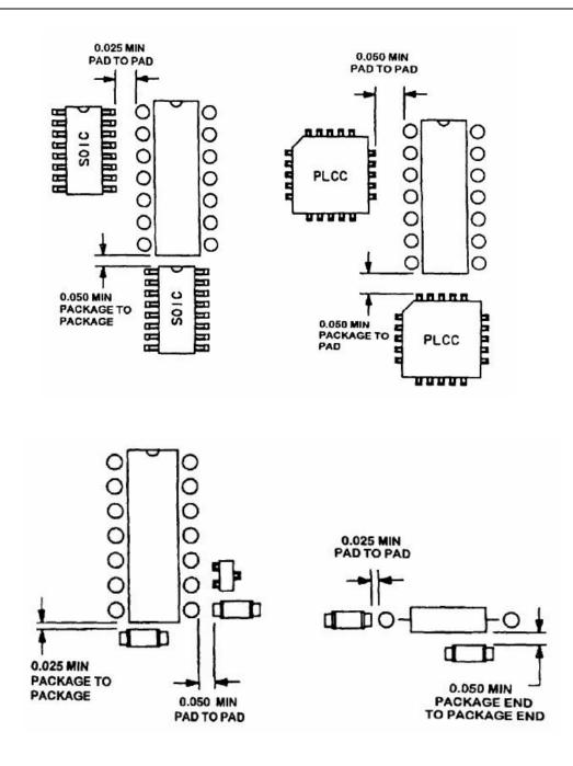
Figure 5-3 SMT TO THRU-PIN COMPONENT SPACING
