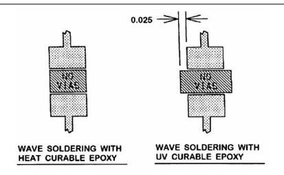
Figure 6-5 VIA PLACEMENT FOR SOLDER SIDE CHIPS
