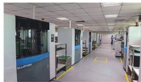
High-speed flying probe machine
