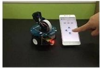
AlphaBot2-Pi robot Bluetooth control
