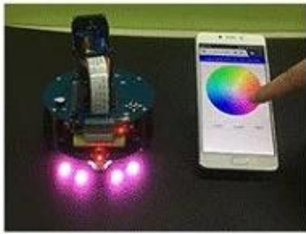
AlphaBot2-Pi robot RGB LED control
