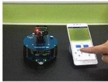
AlphaBot2-Pi robot video monitoring
