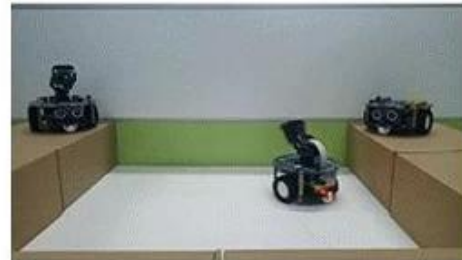
AlphaBot2-Pi robot obstacle avoiding
