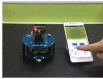
AlphaBot2-Pi robot video monitoring
