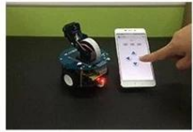
AlphaBot2-Pi robot Bluetooth control
