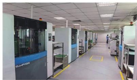
High-speed flying probe machine
