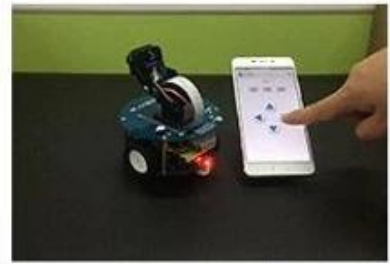
AlphaBot2-Pi robot Bluetooth control
