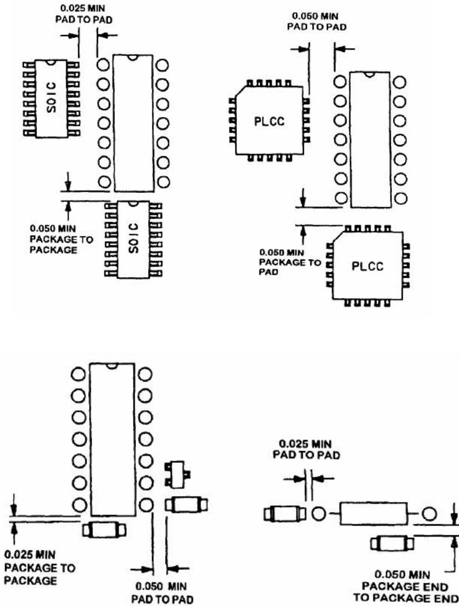
Figure 5-3 SMT TO THRU-PIN COMPONENT SPACING
