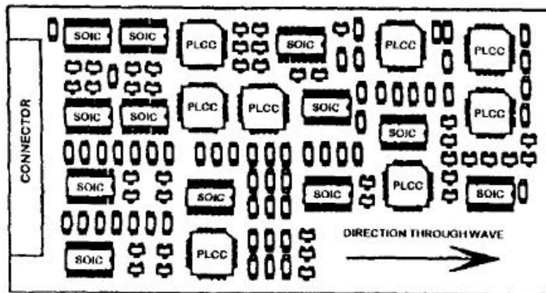
BY SPREADING OUT THE LARGE COMPONENTS EVENLY OVER THE DESIGN, BETTER THERMAL DISTRIBUTION IS ACHIEVED FOR SOLDERING
