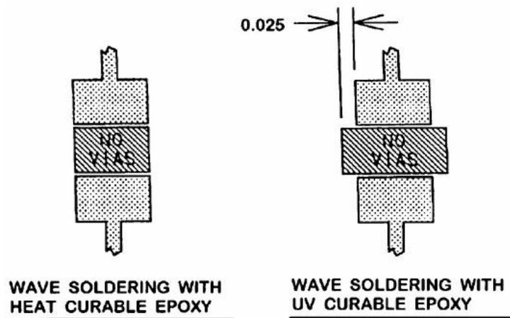
**Figure 6-5 VIA PLACEMENT FOR SOLDER SIDE CHIPS**
