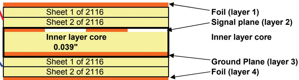
The spacing between the top layer and the signal core would finish at about 9.3 mils
